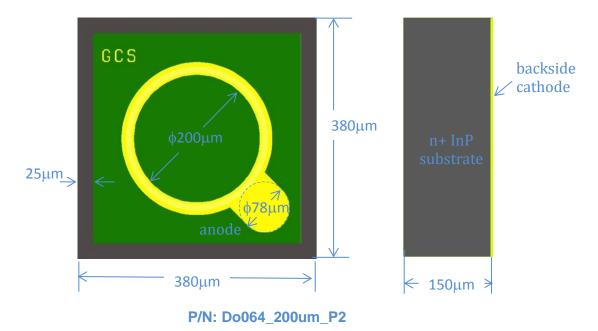
Attention: InP is a brittle material and the device is electrostatic sensitive; observe precaution in handling.
